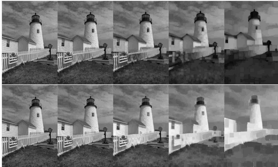
Figure : The effect of the opening (top) and closing (bottom) filters. (Original image is shown on left frame, followed by the filtered image using rectangular windows sized 2x2, 4x4, 8x8, and 16x16.)
